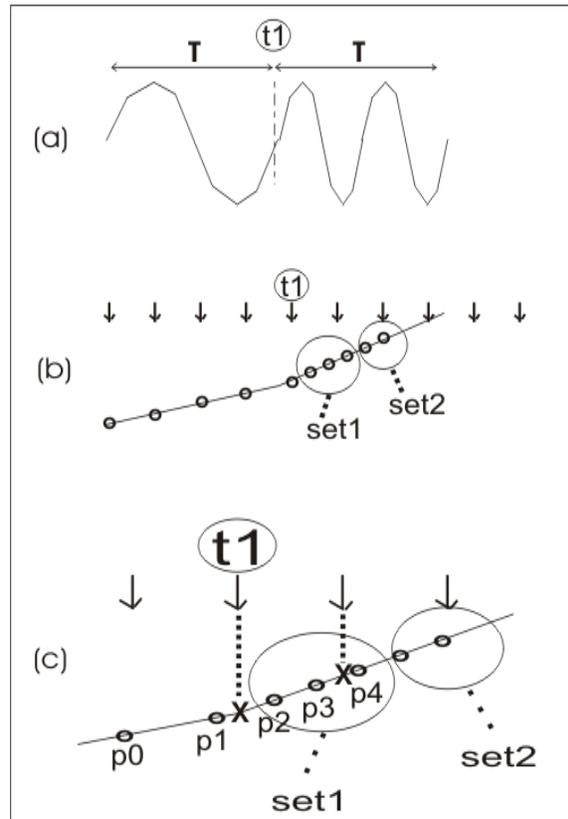
Figure 2. FM operating principle
